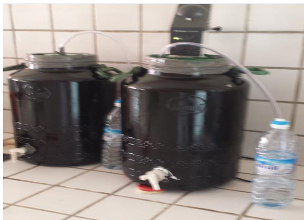
Plate 2. Reactor for methanogenic digestion.
